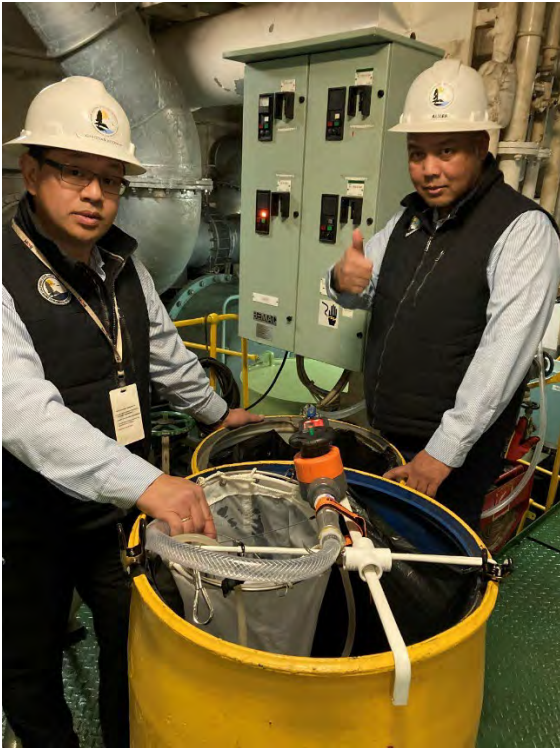
MISIP staff collecting ballast water samples through a plankton net in the engine room of a commercial ship.
