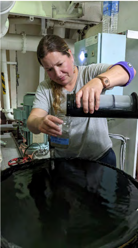
MISIP staff (Lina Ceballos) collecting the contents of a plankton net cod end to capture organisms in a ballast water discharge.
