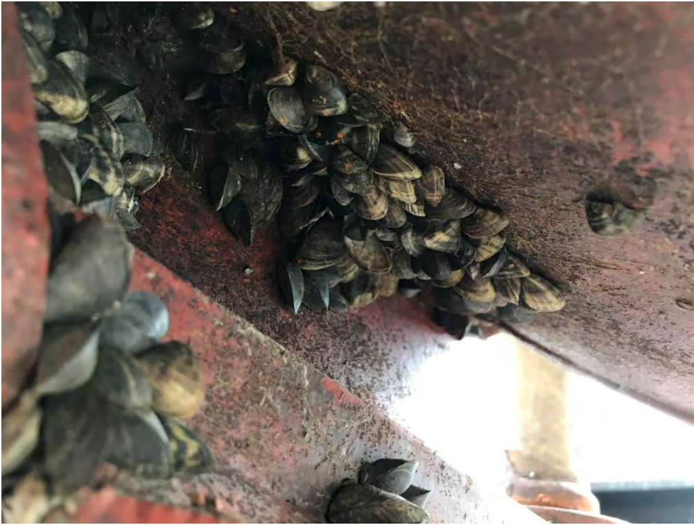
Zebra mussels from the heavily fouled barge that was destined for BC and lab analysis verified that the mussels were viable
