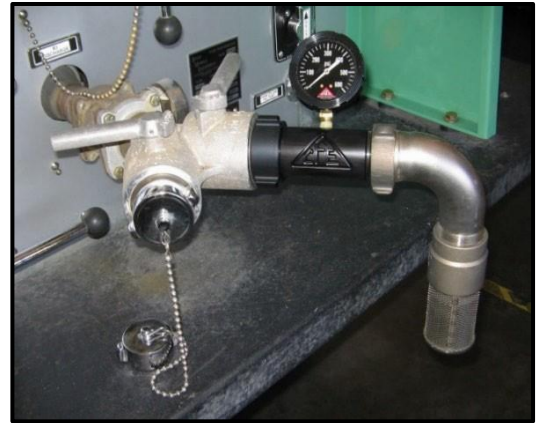
Figure 12: Pressure valve attached to the foot valve
