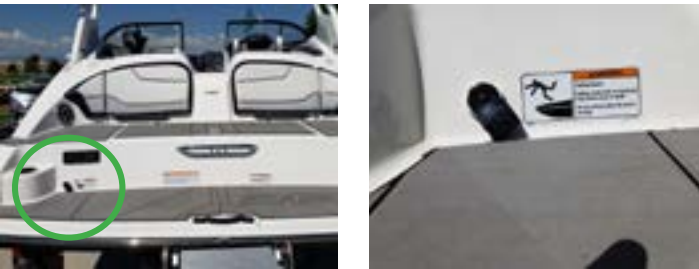
Yamaha 212x Engine Flushing Port Locations
